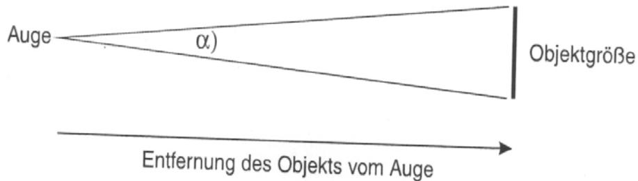
Figure 1.3: Viewing angle  $\alpha$
