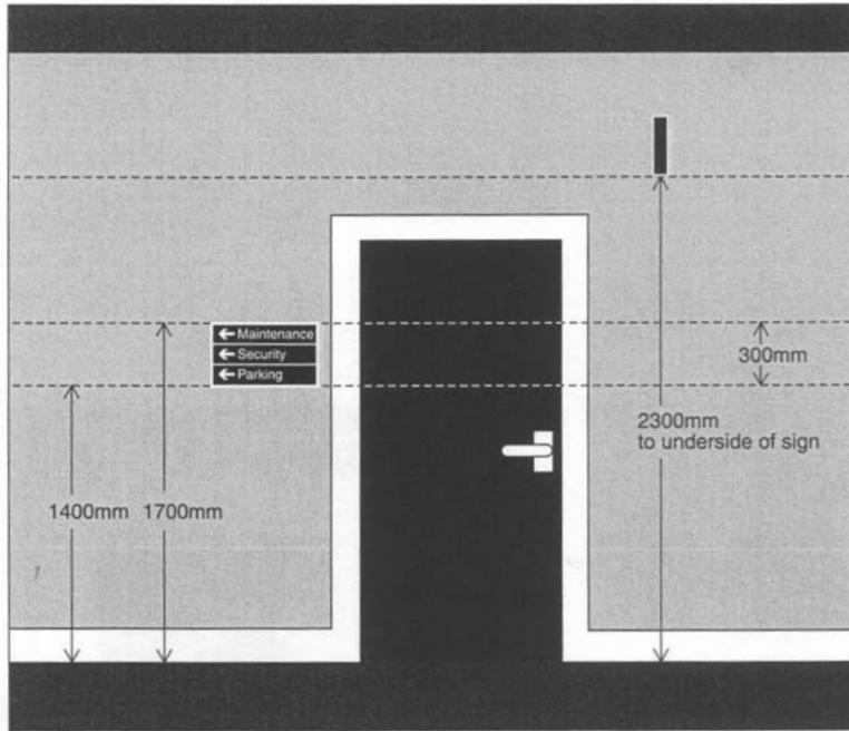
Figure 1.9: Position of signs (Barker et al, 2000)
